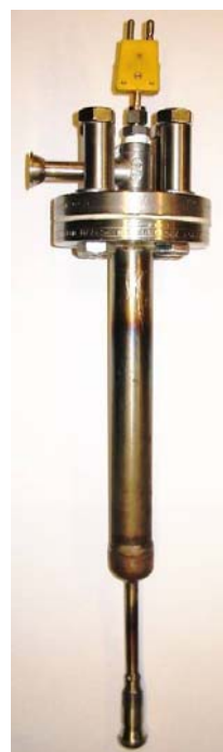
Figure 4-4 Secondary reactor (fixed char bed reactor)
