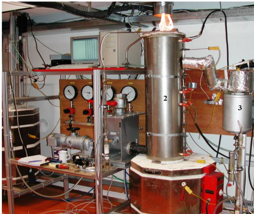
Figure 4-3 Picture of the biomass gasifier and the fixed char bed reactor during one of the experiments, 1. biomass feeder; 2. BFB gasifier; 3. Fixed bed tar cracker
